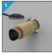
Make sure that the service penetration and the gap are free from dust, dirt and grease. Moisten the structure, if necessary.
