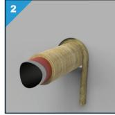
If backing is applied, cut it slightly wider than the gap width and make sure that it is applied to the correct depth in the structure.
